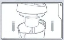
5 Place the lid back onto the jug ensuring it is securely in place.
